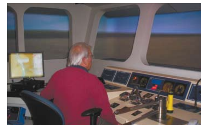
A barge pilot looks out on a simulated river scenario from one of the Seamen's Church Institute's computerized wheelhouses. The simulations help bridge design engineers assess navigability in the vicinity of the new spans based on various environmental conditions.
